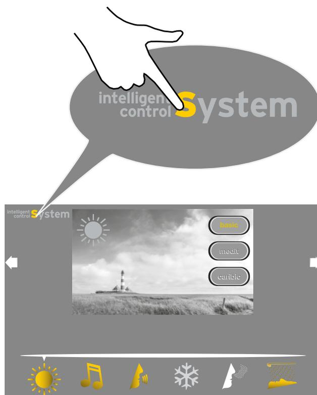
For tanning devices **with** touch display, the standby functions are located on the right side of the service menu start window.
